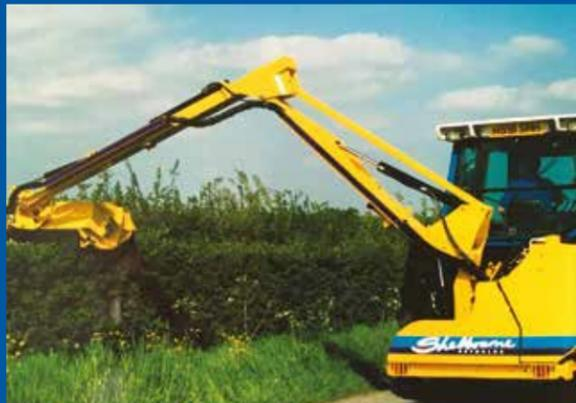
But as hedge trimming rules have changed, resulting in longer intervals that create older, thicker growth, and the importance of verge mowing has increased to meet the need for enhanced road safety, our engineers have kept pace by designing new, higher capacity models.
