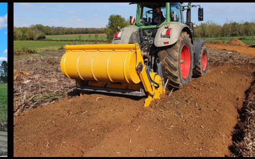
RC65 Deep crushing and soil reclamation
