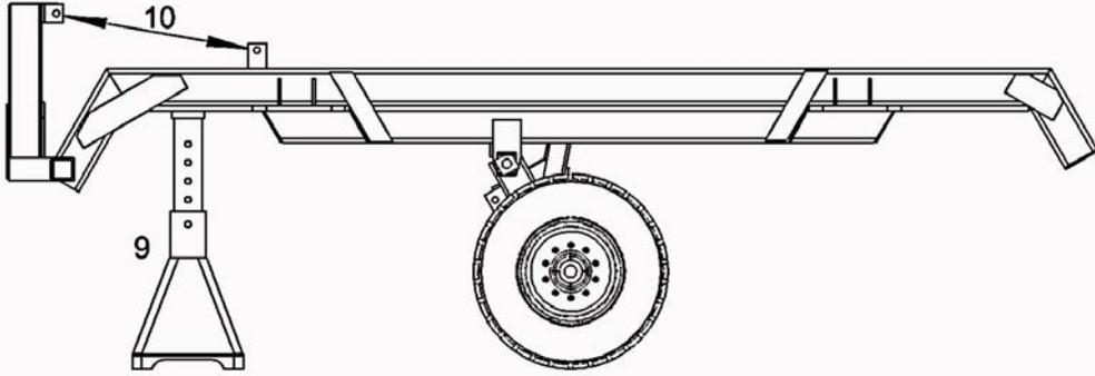
10. If necessary, adjust the chain or strap between the bridle mast and frame cross member to ensure the mast is as vertically straight as possible. This will simplify the installation of the hitch.
