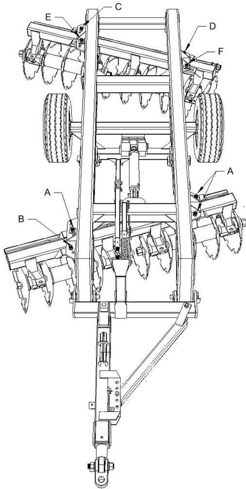
To change the angle of the front gang, loosen the bolts at positions A and remove the bolt at position B. With the disk slightly lowered into the ground, use the tractor to carefully move the disk either forward or backwards to the desired position. Reinstall bolt B and tighten all four bolts to 1500 ft/lbs.
