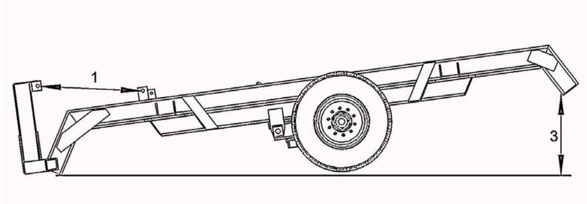
2. Use a chain or strap around the frame and the leg of the transport to keep the transport from dropping when the frame is lifted ( see 3 ). If using a chain, place rubber or matting under the chain to prevent damage to the paint.
