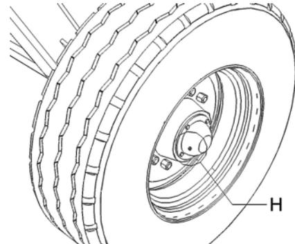
Grease wheel bearings (H) sparingly – six “shots” of grease every 150 hours.
