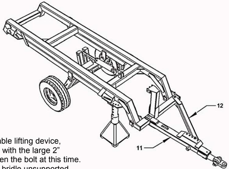
11. Using a forklift or other suitable lifting device, attach the hitch to the bridle with the large 2" fabricated bolt. Do not tighten the bolt at this time. The hitch will hang from the bridle unsupported.
