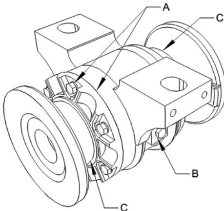
the seals are made of metal, they can expand and contract with extreme temperature fluctuations. When they contract the sealing surfaces separate and small amounts of oil can escape. This will normally occur when the disk is in storage. Putting the disk to use will normally allow the seals to re-seat themselves. Check the oil and add 90W gear oil if necessary.
