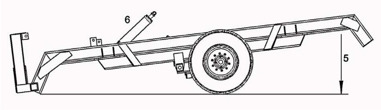
5. Lower the frame to the ground and remove the chain or strap placed in step 2.
