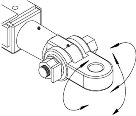
The disk is equipped with a heavy tongue that both flexes and swivels to accommodate the most rugged terrain including large rocks and tree stumps. This is an essential design feature; however it requires extra care when attaching the disk to a tractor.
