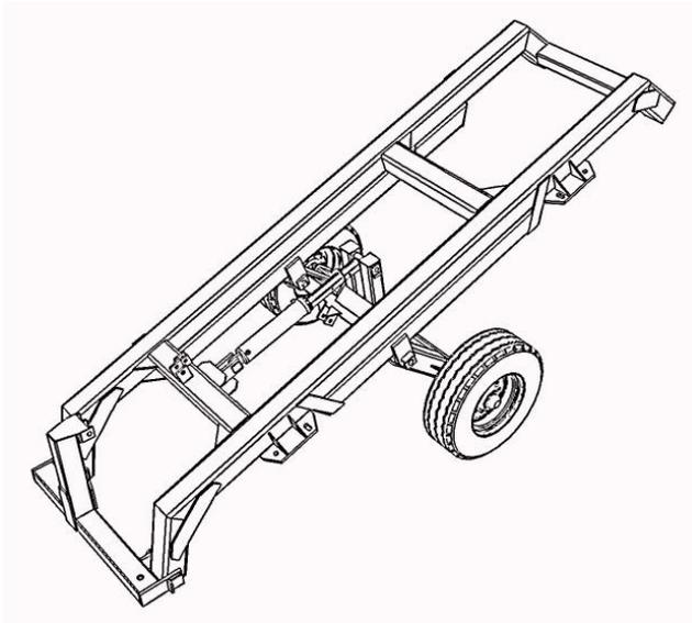
7. By raising and lowering the back of the frame, the transport uprights can be moved until the rod end of the cylinder can be pinned to the transport. Once the cylinder is connected, raise the rear of the disk until the wheels clear the ground. At that point the cylinder should be fully extended.
