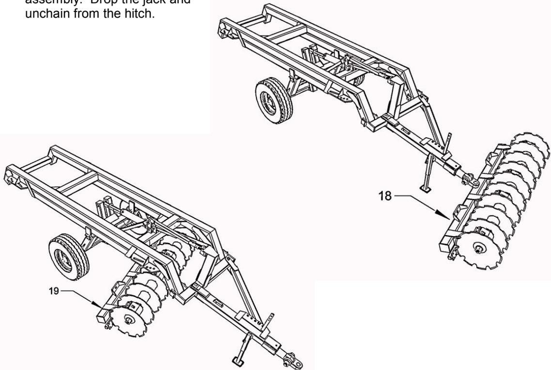
20. Using a single strap or chain of sufficient strength wrapped around the center balance point of the gang bar, lift straight up through the frame. This may require fork extensions or a boomlift. Once a single bolt and nut is installed (do not tighten), the gang bar assembly may be lowered and the chain repositioned to ease installation of the remaining bolts. A pinch bar will make this task easier. Install the bolts as per illustrations 21 and 22 on page 30.
